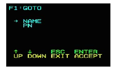
**NAME:** Move highlight bar to "NAME", press [Enter], input name of a port, and then press [Enter] to confirm.
