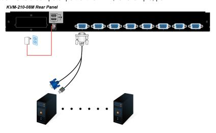
**Step 6.** Attach the power supply to the KVM unit and plug the other end into an electrical receptacle. Now you will see the LED for Port 1 light up. Switch on your monitor from the Port Select button.
