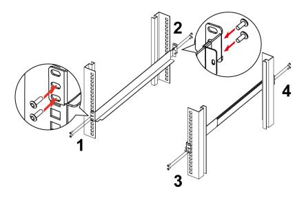
**Step 2.** Slide the switch onto the support flanges. Use the screws supplied with this package to loosely attach the front of the switch to the front of the rack.
