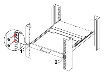
Step 4. Use the screws supplied with this package to attach the bars to the rear of the switch.
